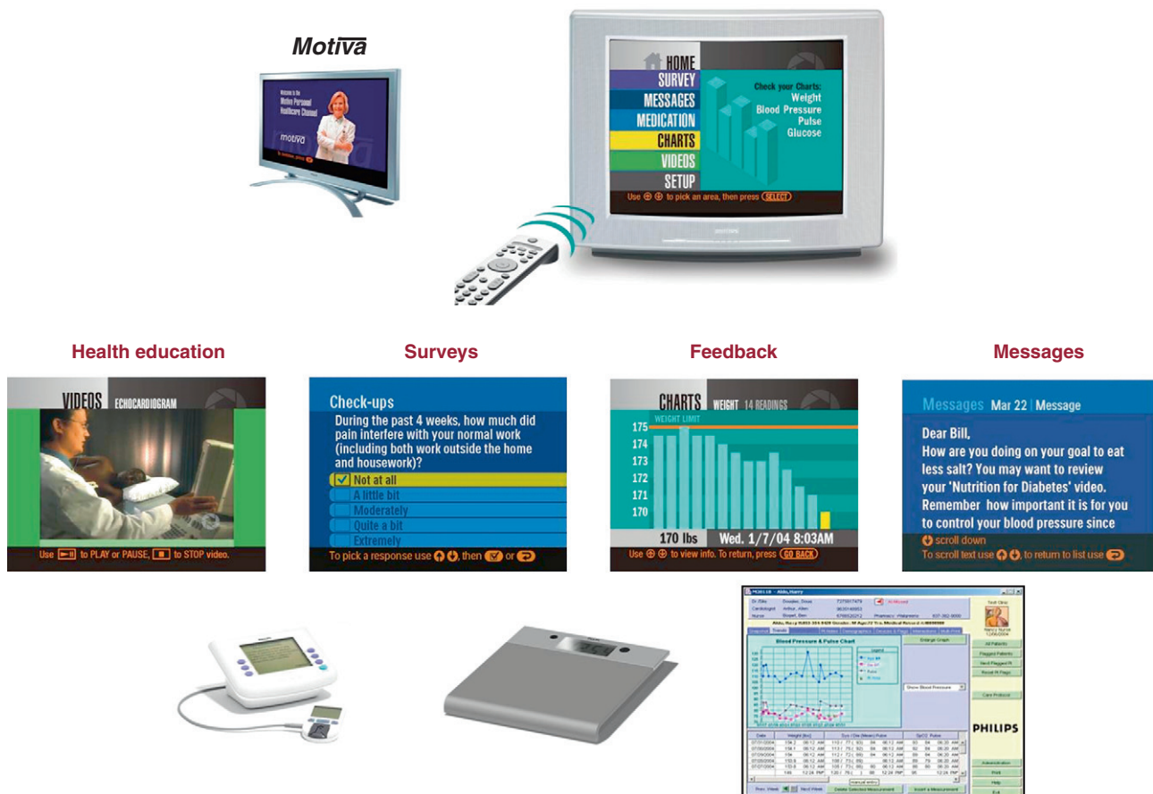
Figure 1. Telemonitoring tools used through a patient's television. The bottom line shows the telemonitoring equipment for weight and blood pressure and a graph of vital signs, as visualized at the heart failure unit workstation.
